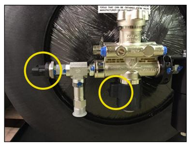
Two connections: HP Sensor and Solenoid
